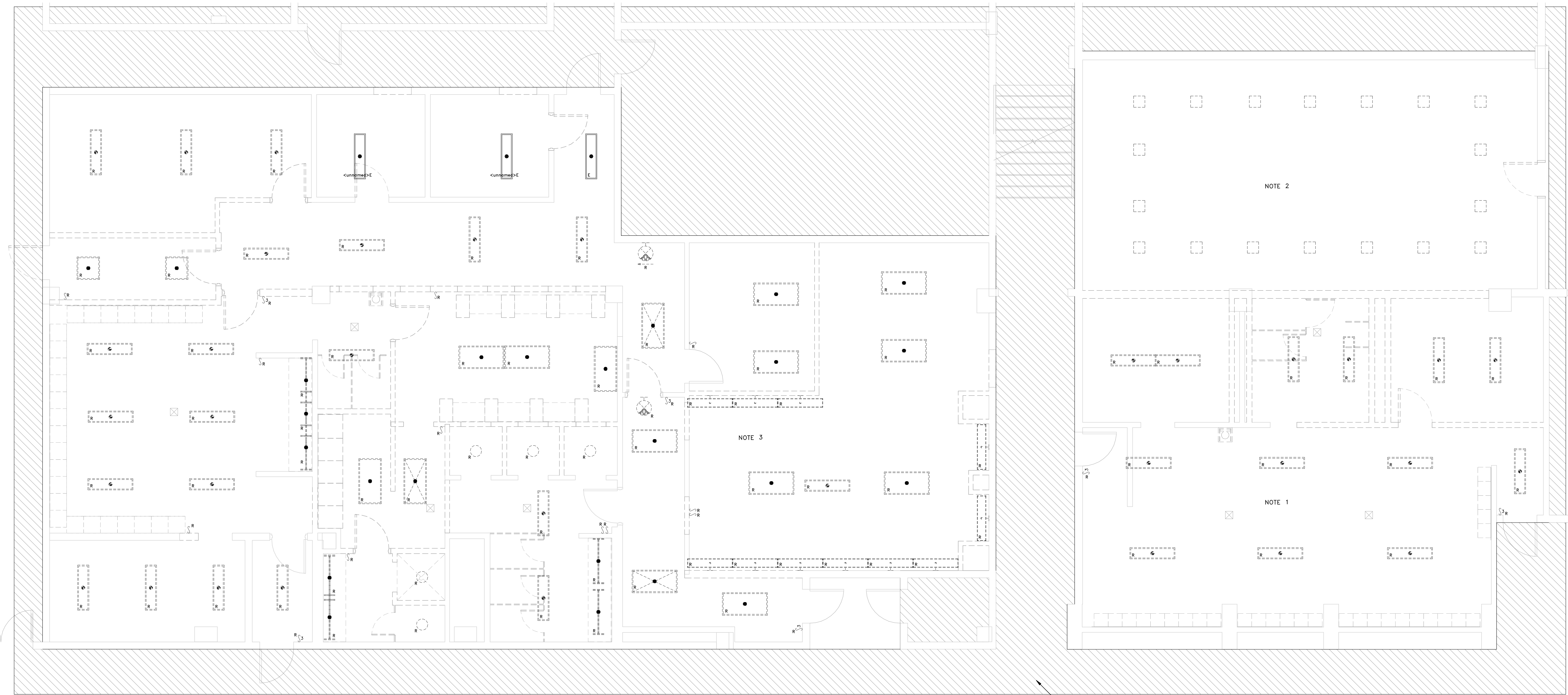
1 FIRST FLOOR LIGHTING DEMOLITION PLAN E1.1 SCALE: 1/4" = 1'-0"
